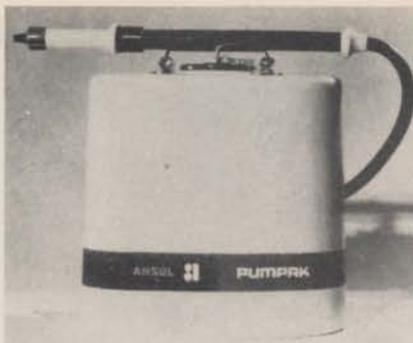
New fiberglass sprayer from Ansul Chemical Co. is said to be up to 40% lighter than comparable metal containers. Self-lubricating plastic slide pump produces a 35-foot stream with a single stroke, and a continuous stream with short, one-third strokes. One-piece nozzle changes flow from wide-angle to long-range stream with slight turn of nozzle tip, company spokesmen reveal. For more information on the new sprayer, write Ansul Chemical Co., Marinette, Wis.
