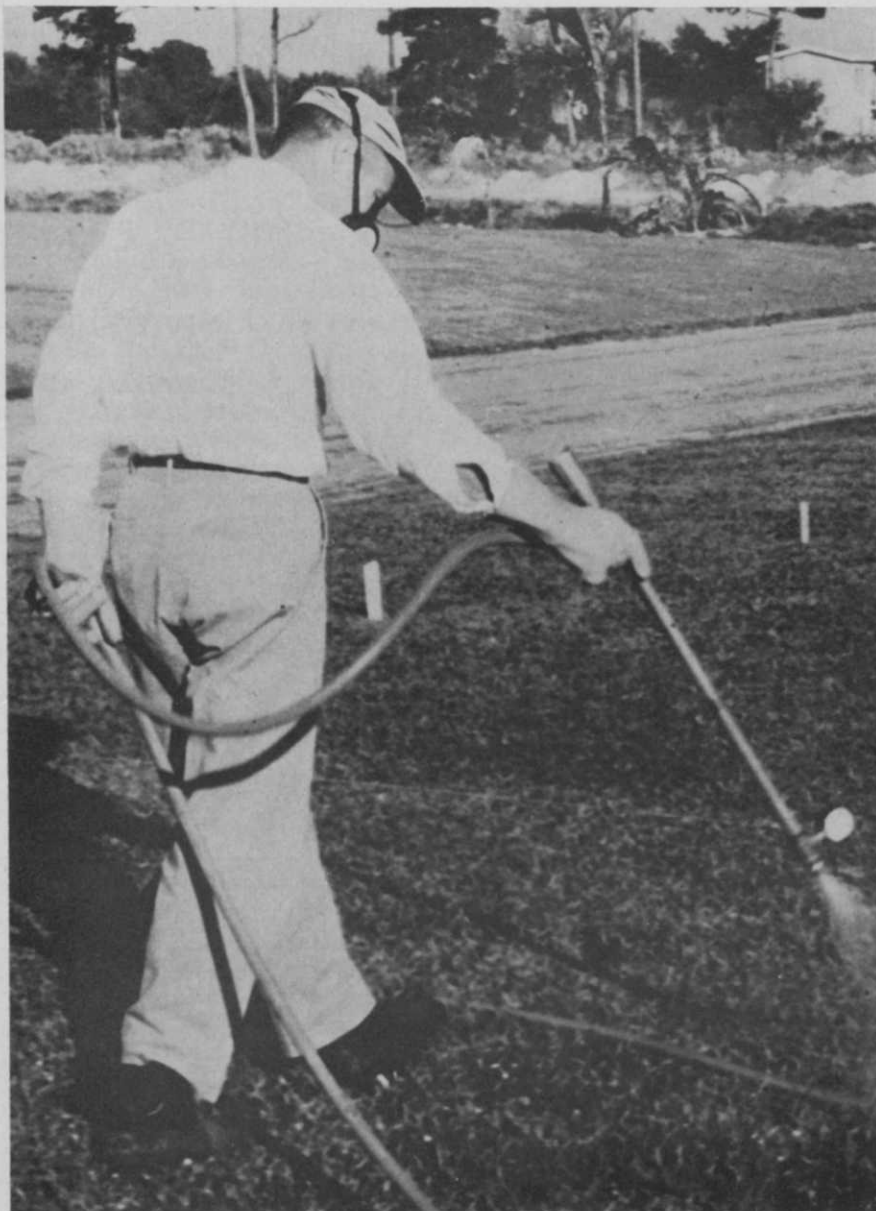
This safety-conscious, masked serviceman is spraying with a homemade gun constructed from galvanized pipe. Note the pressure gauge that is being used for calibration, a necessity when regulating pressure to avoid drift hazard.
