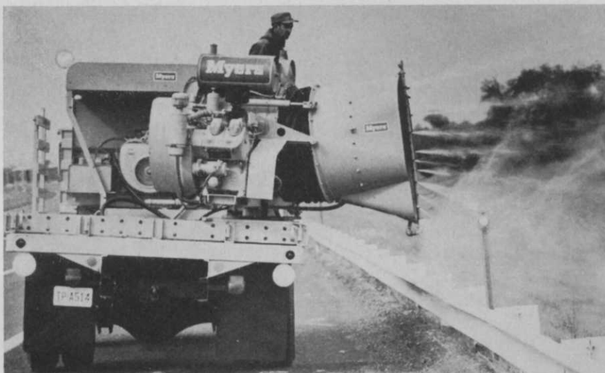
Large, specially built spray rig used for spraying MH-30 on Eastern turnpike was constructed by the F. E. Myers and Bro. Co.
