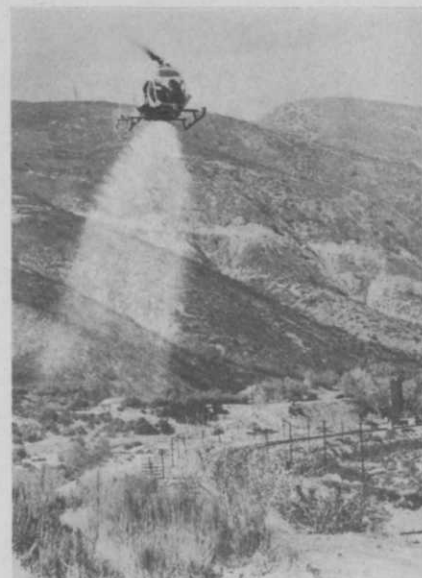
To reduce fire hazards along this California railroad, helicopters spray Ureabor 62, a soil sterilant from U. S. Borax.
