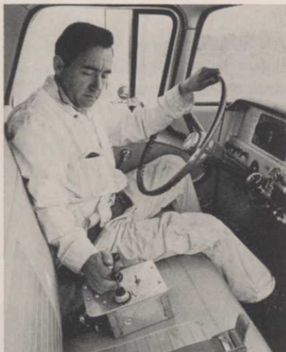
Inside demonstration truck, Naugatuck's Paul Bohne shows how remote controls are used to regulate spray equipment. Note low-speed speedometer mounted outside the cab, just to right of driver's head.
