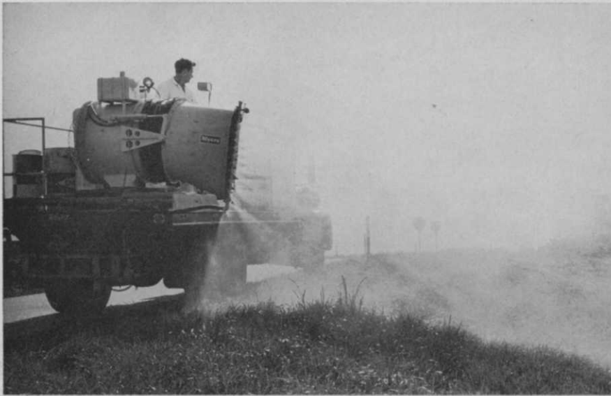
Growth-retarding MH-30 rolls over roadside grass on a North Carolina highway. Naugatuck says about 25,000 acres in 18 states will be sprayed with MH-30 this year in a massive effort to cut the staggering $50 million paid yearly by states to keep roadside grass trimmed.
