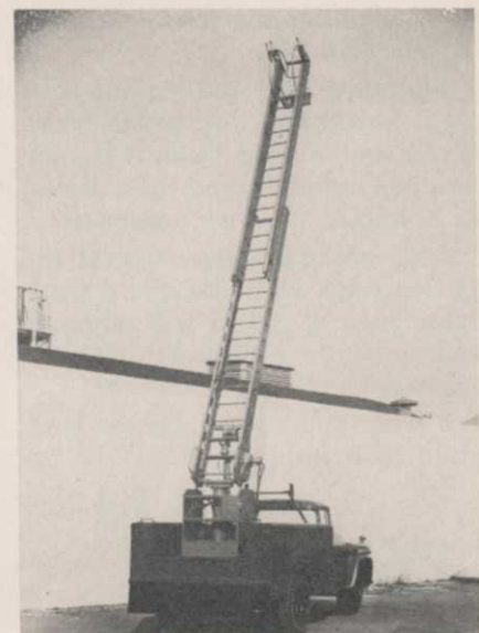
Hydraulically powered aerial ladder from Utility Body Co. rotates in a complete circle, and elevates to 70° angle. Top controls enable CAs to direct ladder while working from it. Utility recommends the device for tree work, as well as allied activities such as bird control. For more information, write the firm at 1530 Wood St., Oakland, Calif.
