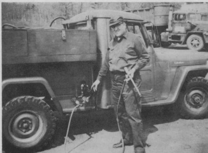
Cost of the war surplus fuel selector valve PCO Bon Pelletier is pointing at was only $3.95. Pressure valve and hose connections are easily accessible.
