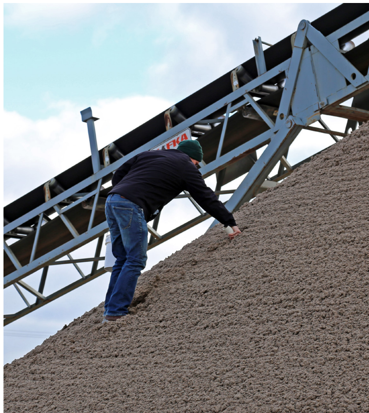
ROOTZONE MIXTURE SAMPLES SHOULD BE COLLECTED AT THE PRODUCTION FACILITY FOR QUALITY CONTROL TESTING.
