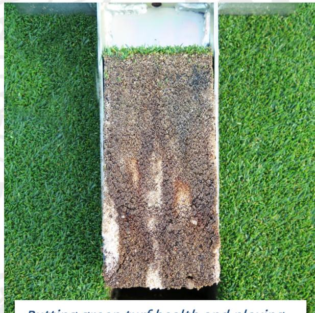
*Putting green turf health and playing conditions were improved by performing regular physical soil tests on the upper 2-3 inches of the soil.*
