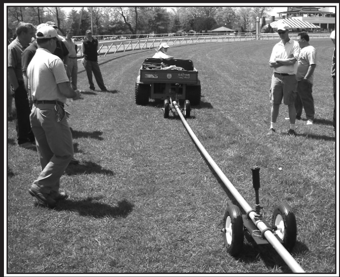
The complexities of irrigating Monmouth Park's oval-shaped thoroughbred turf track and a fixed inside rail necessitate the use of an innovative towline irrigation system.
