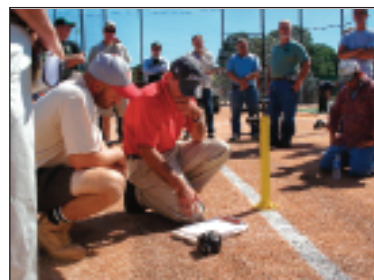
Joel Taylor (l) and Brad Park (r) assess surface hardness values generated by the Clegg Impact Soil Tester on the Recchino Field Complex synthetic infill field.
