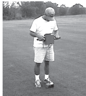
A Remik CP-20 cone penetrometer was used to measure the resistance of soil to the insertion of a probe.
