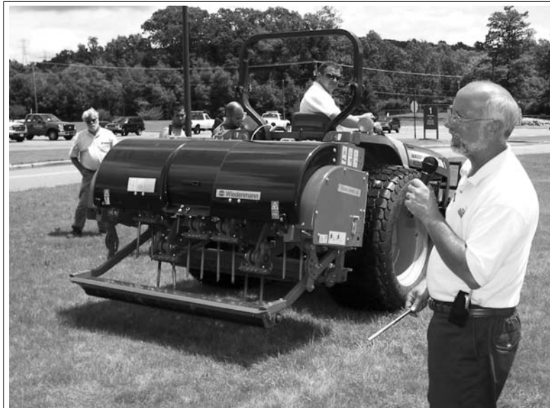
Dennis DeSanctis, Aer-Core, Inc. describes a Wiedenmann deep tine aerification unit.
