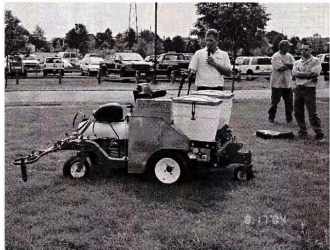
Gregson Clark spraying Equip Hylander Self-Propelled Turf Applicator
