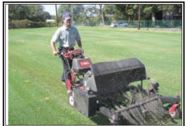
A new machine equipped with rubber paddles has been developed at Rutgers University to uniformly apply wear to turfgrass variety trials. Both operating speed and paddle rpm can be controlled with this unit. It will be demonstrated as part of the SFMANJ Spring Field afternoon session at Rutgers Hort, Farm II on April 12, 2007.
