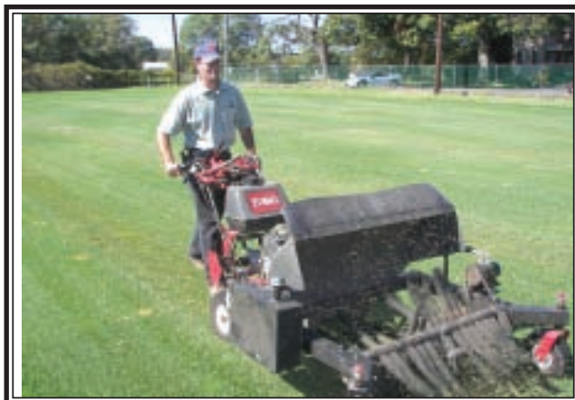
A new machine equipped with rubber paddles has been developed at Rutgers University to uniformly apply wear to turfgrass variety trials. Both operating speed and paddle rpm can be controlled with this unit. It will be demonstrated as part of the SFMANJ Spring Field afternoon session at Rutgers Hort, Farm II on April 12, 2007.
