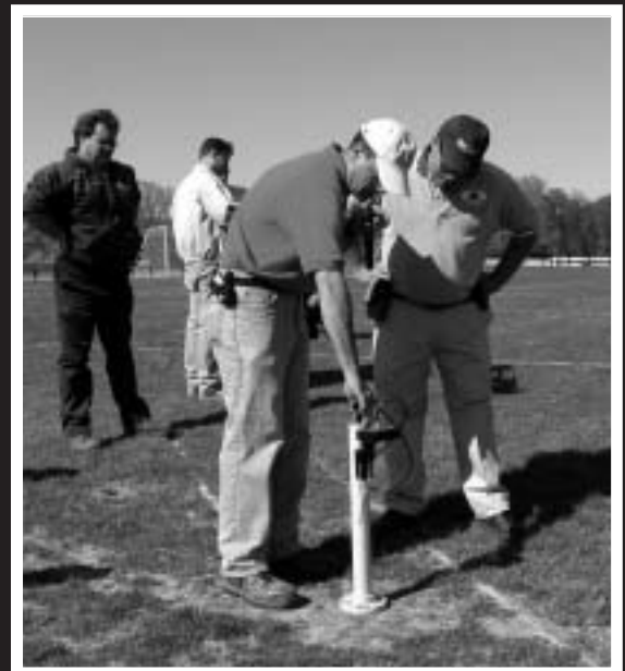
Brad Park demonstrates the use of the Clegg Impact Soil Tester to Don Savard, CSFM, CGM, and other attendees at the SFMANJ District I meeting held at Harrington Park, Long Valley, NJ on May 4, 2006.
