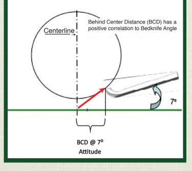
Figure 2. This diagram represents an example of a less aggressive cutting unit. The red arrow indicates a flatter angle of clip. Notice the BCD distance is now closer to the reel centerline.
