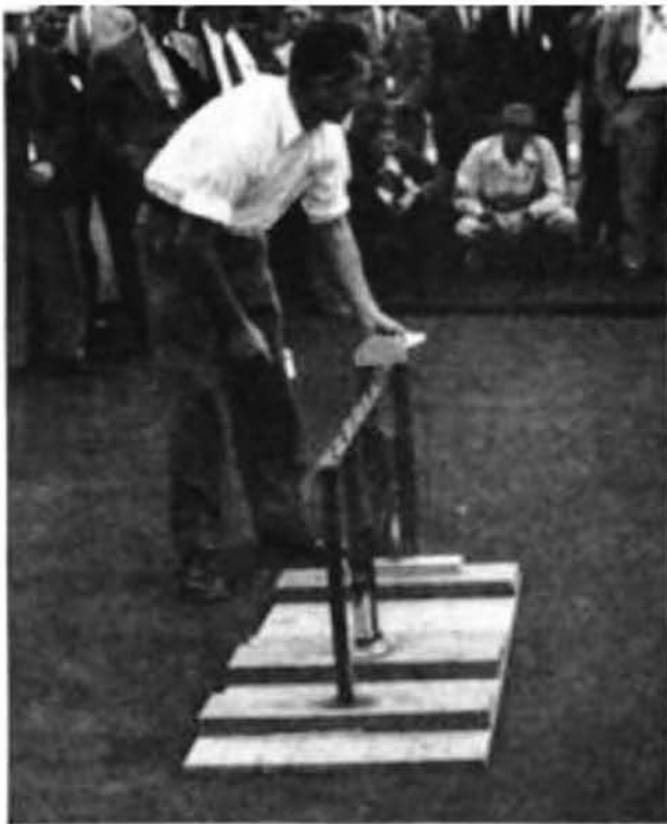
Charles H. Allen demonstrates compressometer which he designed at R. I. Agricultural Experiment station to measure springiness of turf.
