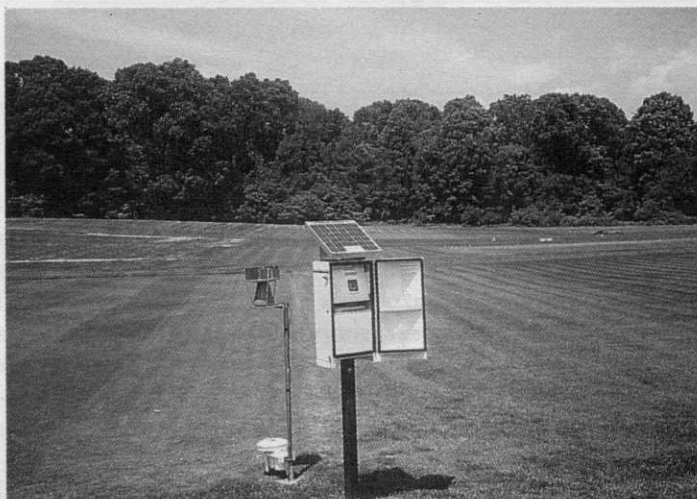
Fig. 3. Commercially-available weather station with built-in pest prediction models or pest alert programs.
