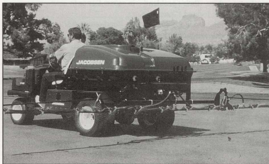
Advances in spraying equipment have enabled superintendents to reduce the amount of fungicide applied while maintaining effective disease control. Photo courtesy: Smithco.
