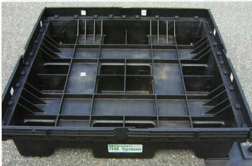
GreenTech ITM modules have channels 22 in. apart on all four sides. The channels allow modules filled with growing turf to be moved via forklift. They also create a drainage network. Irrigation water quickly drains through holes in the bottom of each module to prevent saturation.
