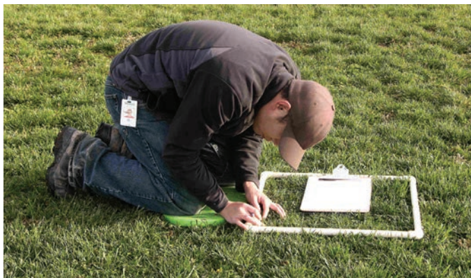
Figure 5. Point quadrat used to estimate percent species cover in plots.
