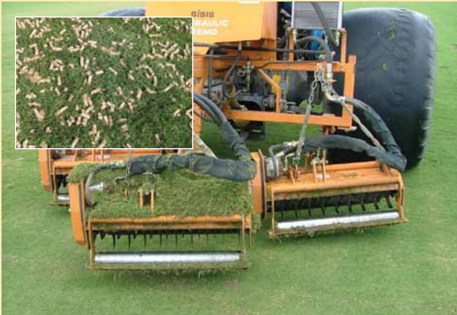
Above. Material collected as a result of vertical mowing. Inset. Cores from aeration done to improve soil compaction on an athletic field (photo courtesy of Eric Lyons).
