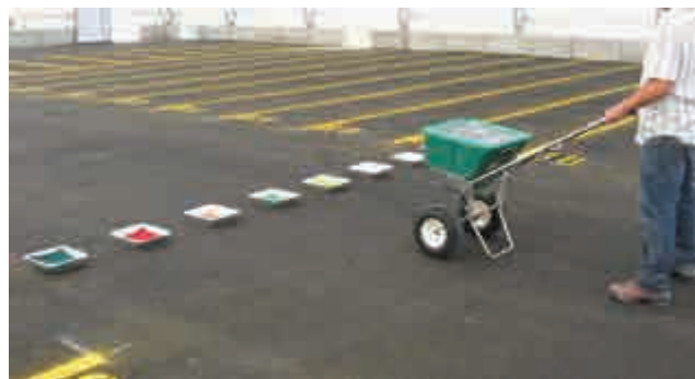
Figure 2. Evenly spaced pans to either side of path of travel (photo courtesy of Ferti Technologies)
