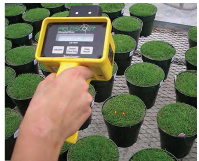
Figure 5. Spectrum FieldScout chlorophyll meter.
