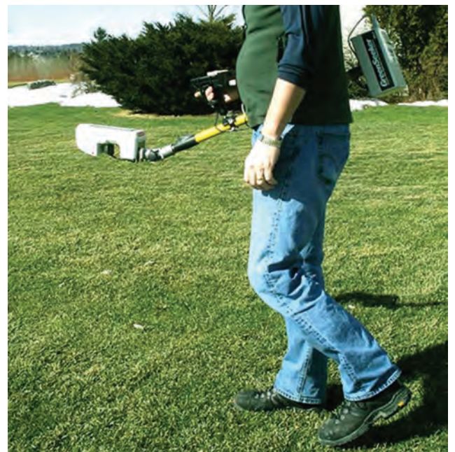
Figure 4. Greenseeker canopy reflectance sensor system.
