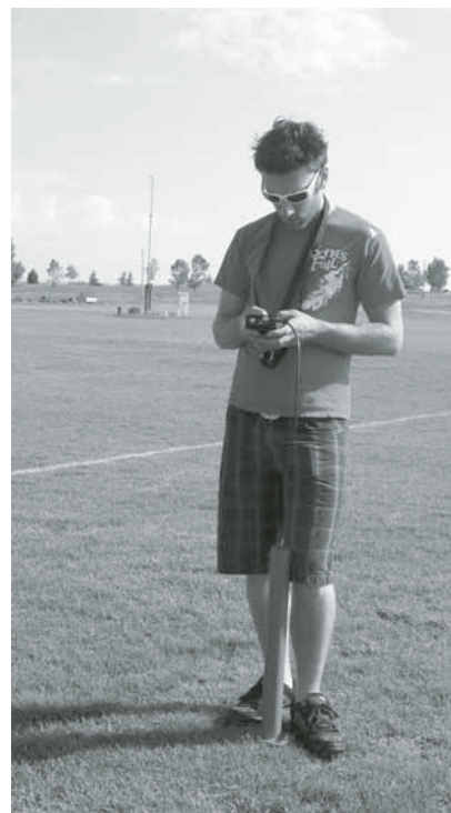
Above: Measuring surface hardness with a Clegg Hammer.
