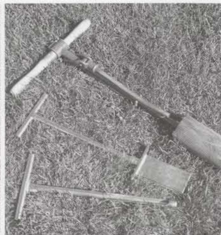
Figure 3. Sampling tools: cup changer (top), slab sampler (middle), soil probe (bottom).
