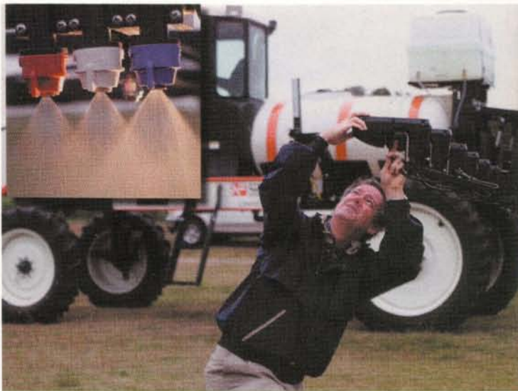
Optical sensors assess nitrogen deficiencies and spray fertilizer where needed. Picture courtesy of NTech Industries, Inc. and Oklahoma State University (published in CAAR Communicator, Dec. 2001, Vol. 22, No. 5).
