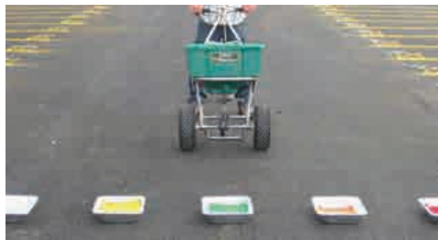
Figure 1. Spreader alignment for pan test (photo courtesy of Ferti Technologies)
