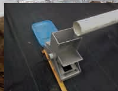
Figure 3. Tipping bucket used to measure water volume from leaching and runoff and plastic container used to collect water sample.
