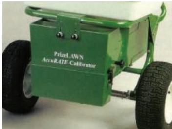
Figure 4. A common calibration catch used for pedestrian broadcast spreaders (photo courtesy of White Castle)
