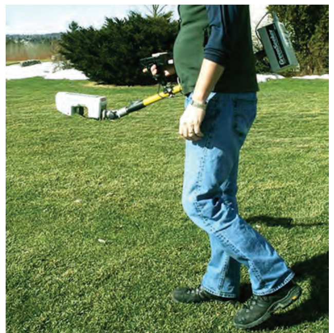
Figure 4. Greenseeker canopy reflectance sensor system.
