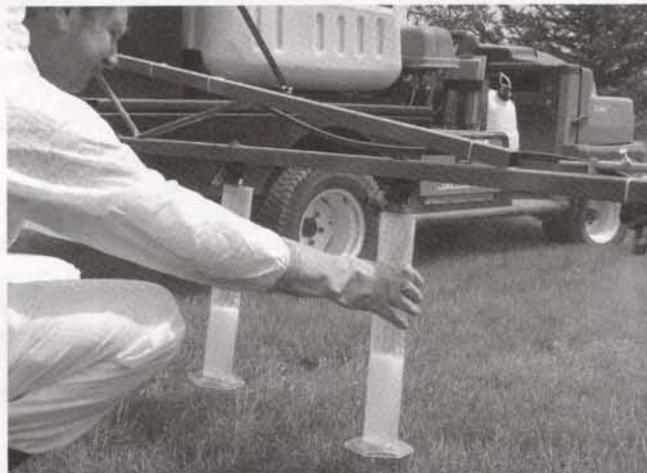
be replaced. While you are doing the calibration on your sprayer take note of the nozzle spray patterns. Each nozzle should have a uniform spray pattern without heavy streaks or skips. Nozzles with distorted spray patterns should be replaced.
