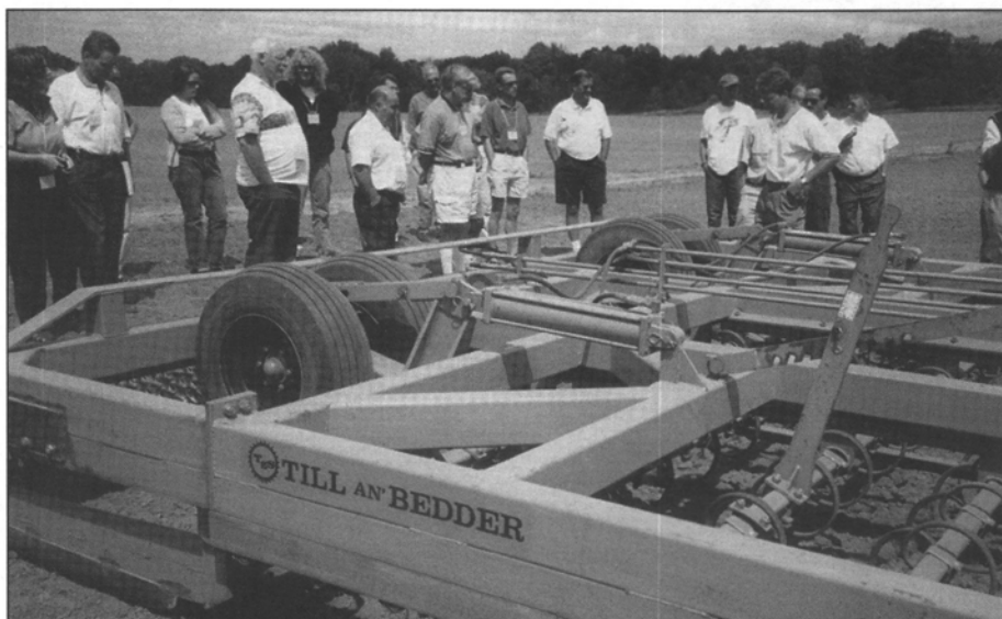
The Schmeiser tiller and bedder used at Compact sod farms to cultivate and firm the land area prior to seeding.
