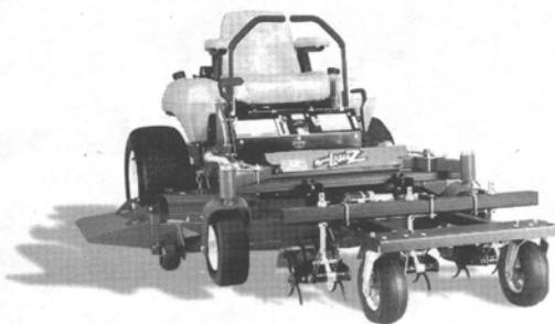
The JRCO aerator fits commercial walk behind and riding mowers. The 38-inch-wide unit can aerate 66,000 square feet per hour at 5 mph. Aeration holes are up to 3 inches deep, and the unit dispenses loose plugs of soil, not hard core plugs. There is no subsurface compaction around or at the bottom of the holes, which promotes water and air filtration. Video available showing this and other mower attachments.
