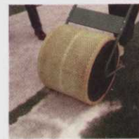
10:07 a.m. Pick up residue. (Recommended to reduce buildup in infill, but rinsing okay)
