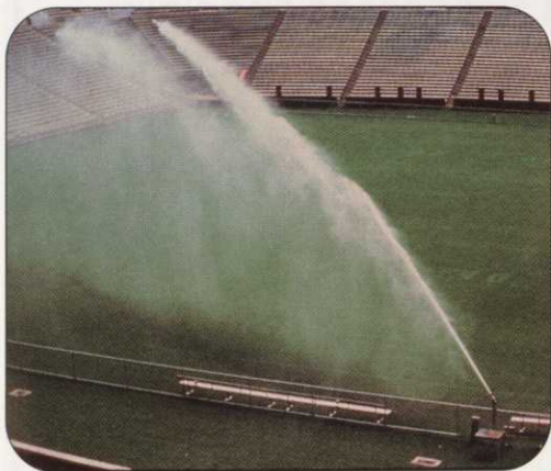
Off-field irrigation gun in use
