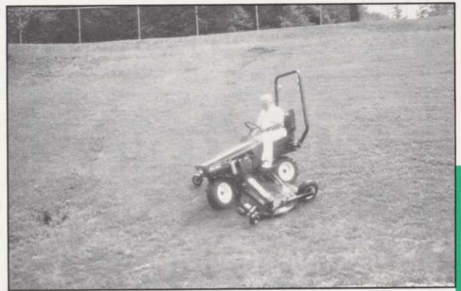
Harry Gill, Milwaukee County Stadium, tries out a new mower at Eastern Sports Turf Institute. The mower is designed for severe slopes and banks.
