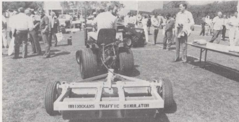
Dr. Matt Leonard, University of California Riverside, demonstrating wear tolerance traffic simulator.
