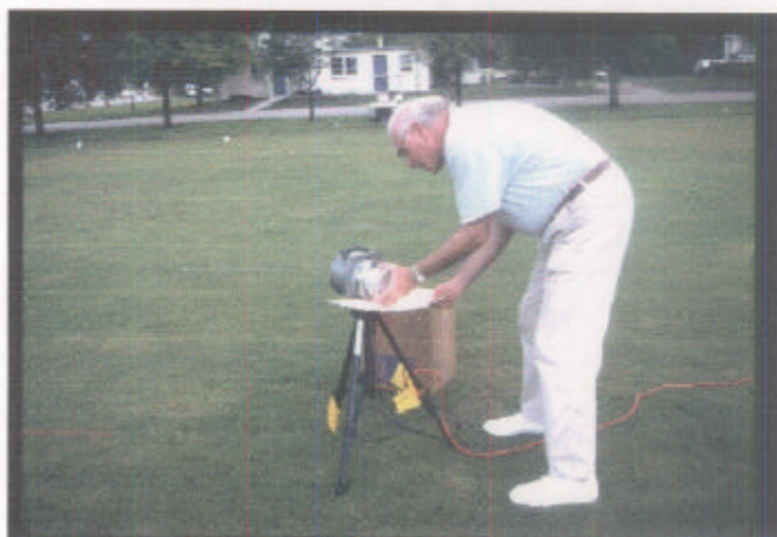
Mr. David Rich, Chemist, emptying XAD-4 resin used to adsorb air-borne pesticide from an air sampler during a pesticide volatilization experiment.
