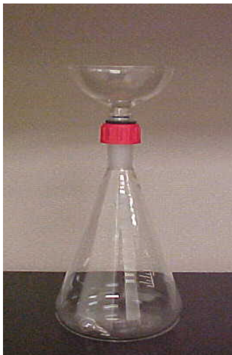
Custom made bottle designed to collect first flush water samples from fairways.
