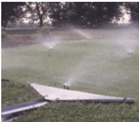
Plots were constructed at the University of Illinois to study how timing of irrigation following pesticide application can reduce runoff.
