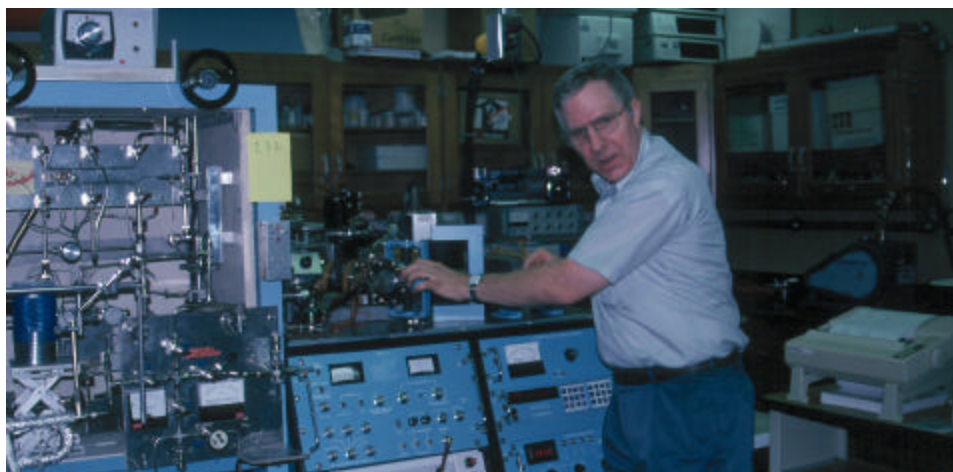
At the University of Illinois, Dr. Richard Mulvaney has developed a specialized mass spectrometer to measure NO 2 gas volatilized from labeled nitrogen fertilizer.
