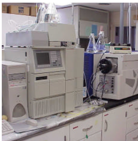
After each event, water was collected from each plot and analyzed by high pressure liquid chromatography for residual insecticide or herbicide.
