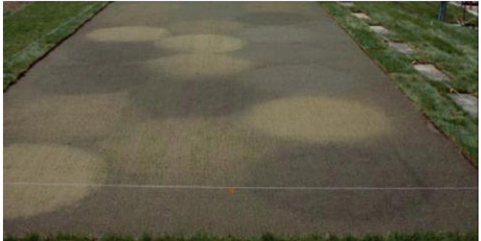
Researchers constructed a series of replicated, enclosed rootzones to measure the effects of rootzone depth and composition on the water use rate of putting greens.
