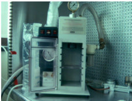
The biolistic gun is used to shoot DNA-coated gold or platinum particles into embryogenic callus tissue.
