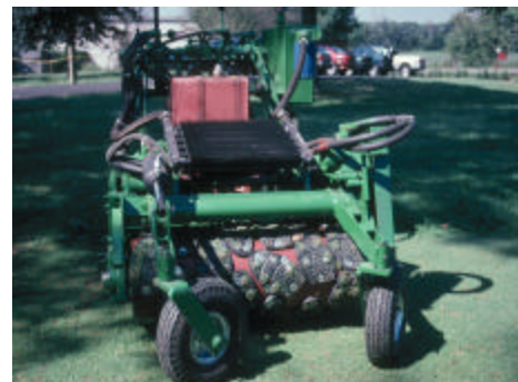
Dr. Bill Meyer has created a traffic machine with spikeless golf shoe soles for screening cool-season grasses at Rutgers University.
