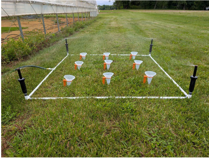
Figure 3. Calibration of an irrigation square utilized for single plot irrigation in the water use trial (study 3).
