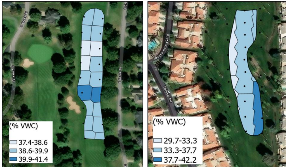
Figure 3. Example of hydrozone delineations on two golf course fairways based on volumetric water content (% VWC). The left fairway (Kentucky) uses individual-head control, resulting in smaller and more discrete hydrozones, whereas the right fairway (California) uses block-based irrigation, leading to larger grouped hydrozones. An in-ground soil moisture sensor will be installed within each hydrozone to monitor conditions and trigger irrigation at the zone level.
