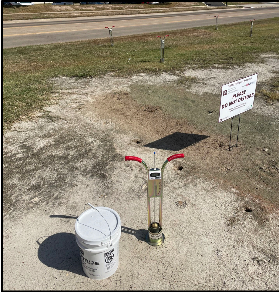
Figure 5. Image of a sodium degraded area selected for the re-establishment study at the TAMU location. The double ring infiltrometers show the approximate areas where the soil chemical/physical characterization samples were obtained.
