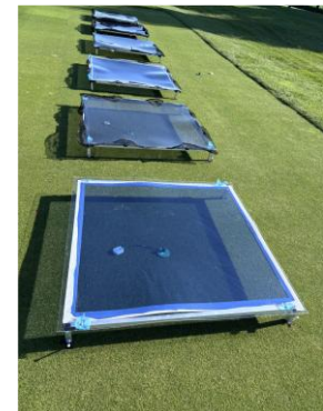
Figure 1: Photoselective filters and shade cloth taped under plexiglass
