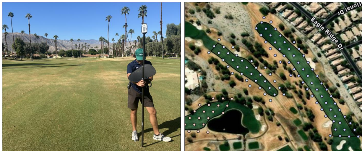
Figure 1. Georeferencing sprinkler locations at Monterey Country Club in Palm Desert, California (left), and mapped sprinkler heads and fairway boundaries at TPC Summerlin in Las Vegas, Nevada (right).
