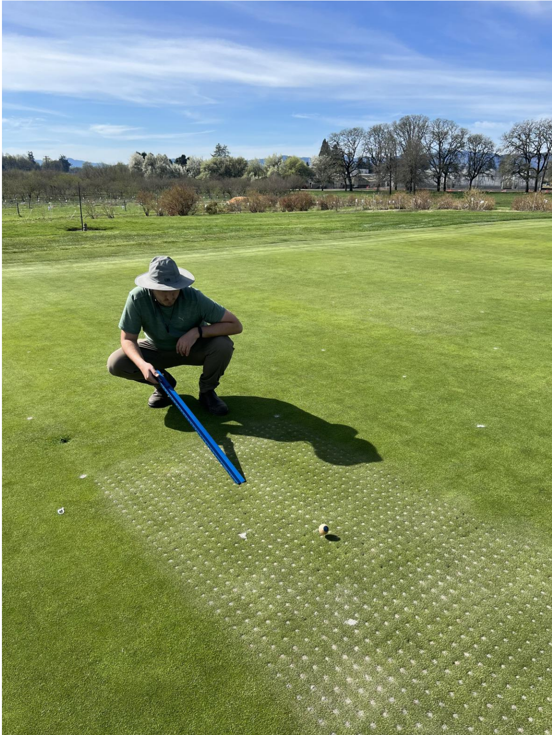
Image 2. Collecting ball roll distance (green speed), smoothness, and trueness with the USGA GS3 ball; Oct 2025.
