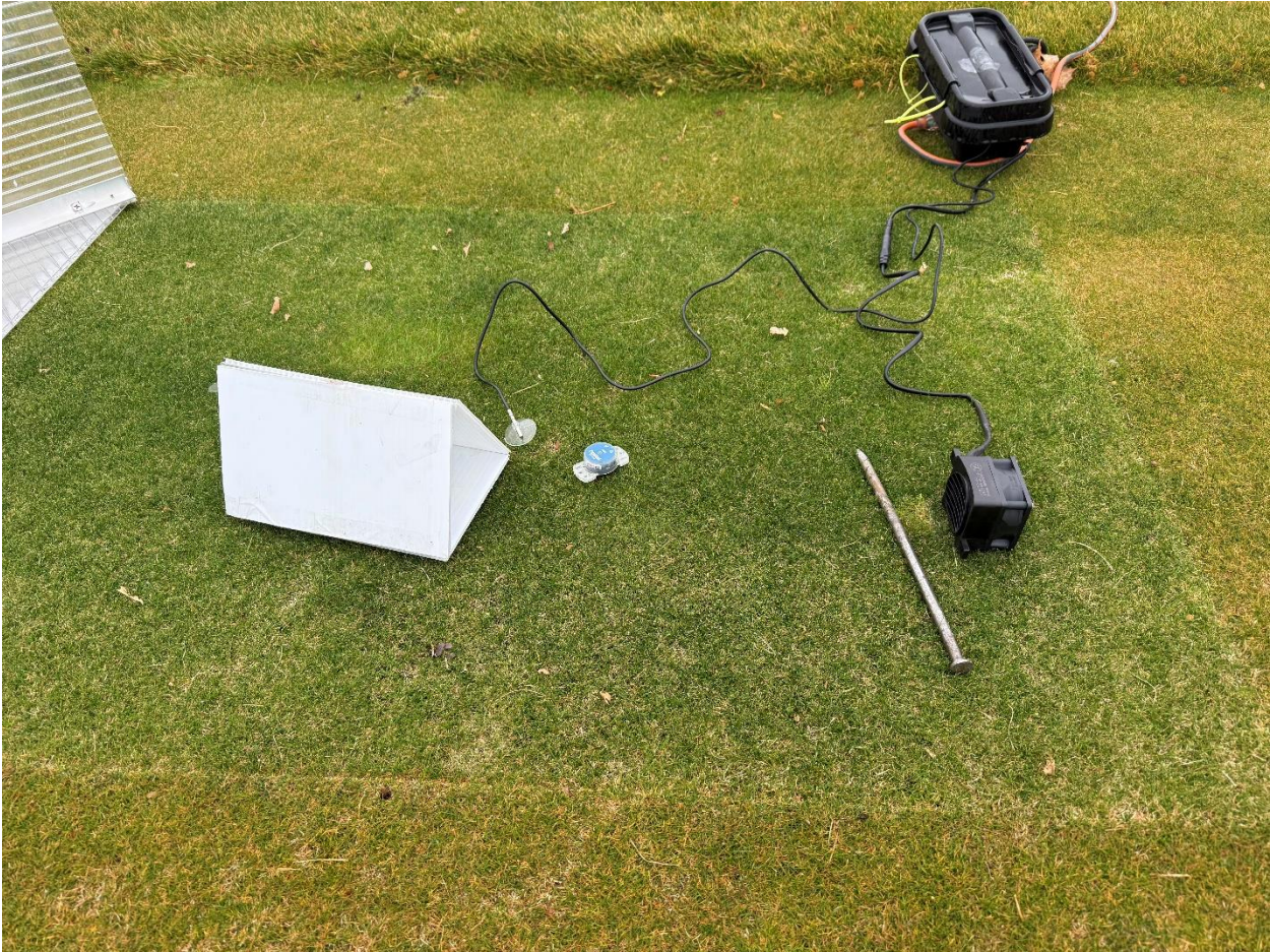
Figure 4. A radiation shield, thermostat probe, Bluetooth temperature logger and small heater placed under A-frame greenhouses to maintain a warmer air temperature to thaw out the soil surface.
