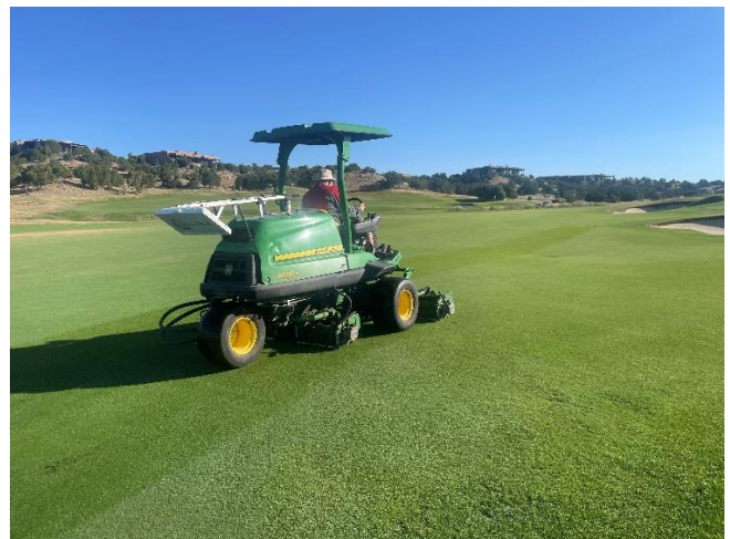
Figure 3. turfRad sensor scanning #16 with a Utility Vehicle (left) and with a fairway mower (right).
