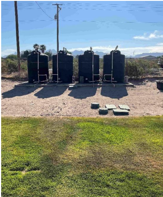
Figure 1. Four water tanks containing tap water (Control), water high in bicarbonate, water high in bicarbonate with N-pHuric, and water high in bicarbonate with WaterSOLV™ Curative (left to right).
