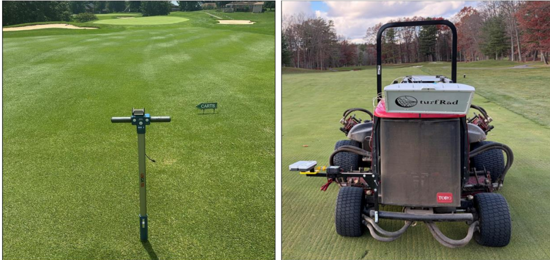
Figure 2. Handheld soil moisture sensor data collection on fairways at Frankfort Country Club in Kentucky (left), and mower-mounted PoLRa and VI sensors used for fairway scanning at Toftrees Golf Resort in Pennsylvania (right).
