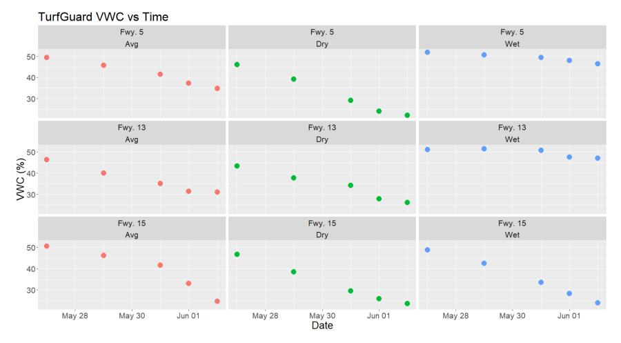
**Figure 4.** Mean, daily TurfGuard percent volumetric water content (VWC) of each moisture class (Avg = moderate, Dry = low, Wet = high) of fairways receiving the SMS-based irrigation treatment during a dry down event from May 27 – June 2, 2020 at Edina Country Club.
