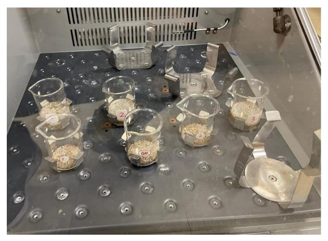
Figure 3. Lab mixed samples with pre-determined percentage organic matter on an incubator shaker (New Brunswick Scientific, Edison, NJ 08817)
