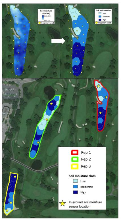
**Figure 2.** Top-left, percent volumetric water content (VWC) on one fairway in the soil moisture sensor treatment; top-right, soil moisture classes within delineated management zones on one fairway in the soil moisture sensor treatment; bottom, in-ground soil moisture sensor locations within each soil moisture class on the fairways receiving the SMS-based treatment.
