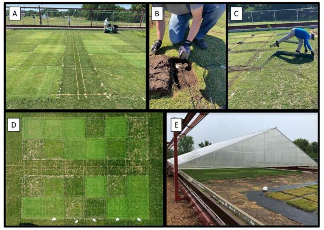
Figure 1. Plots in the dry down experiment in St. Paul, MN. A) following installation of soil moisture sensors; B) installing a CS655 soil moisture sensor; C) installing aluminum barriers between plots to discourage lateral water movement; D) overhead view of plots 15 d into first dry down; E) rainout shelter covering the dry down plots during a precipitation event.
