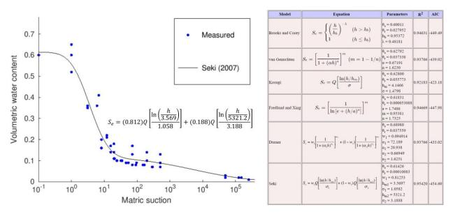
Figure 2. Combined soil water retention data for samples collected from plots in the dry down experiment. A Seki model provided the best fit of the data based on AIC and  $R^2$  values where *h* is the matric potential, Q is the complementary cumulative normal distribution function, and  $S_e$  is the calculated effective saturation.
