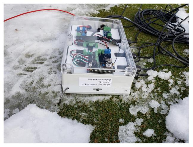
Figure 2. Sensor nodes installed and buried under an inch of ice at the University of Minnesota's Turfgrass Research, Education and Outreach Center. Photo credit: Andrew Hollman.
