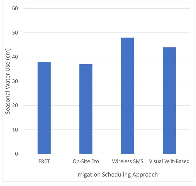
**Figure 2**. Mean seasonal water use for each irrigation scheduling treatment. Data were derived from difference between water meter readings at trial initiation and end of season, and are pooled across the 2019-2020 seasons.
