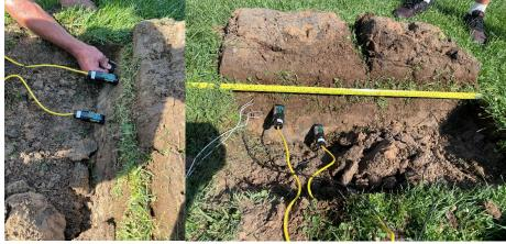
Figure 5: Installation of soil moisture and temperature sensors
